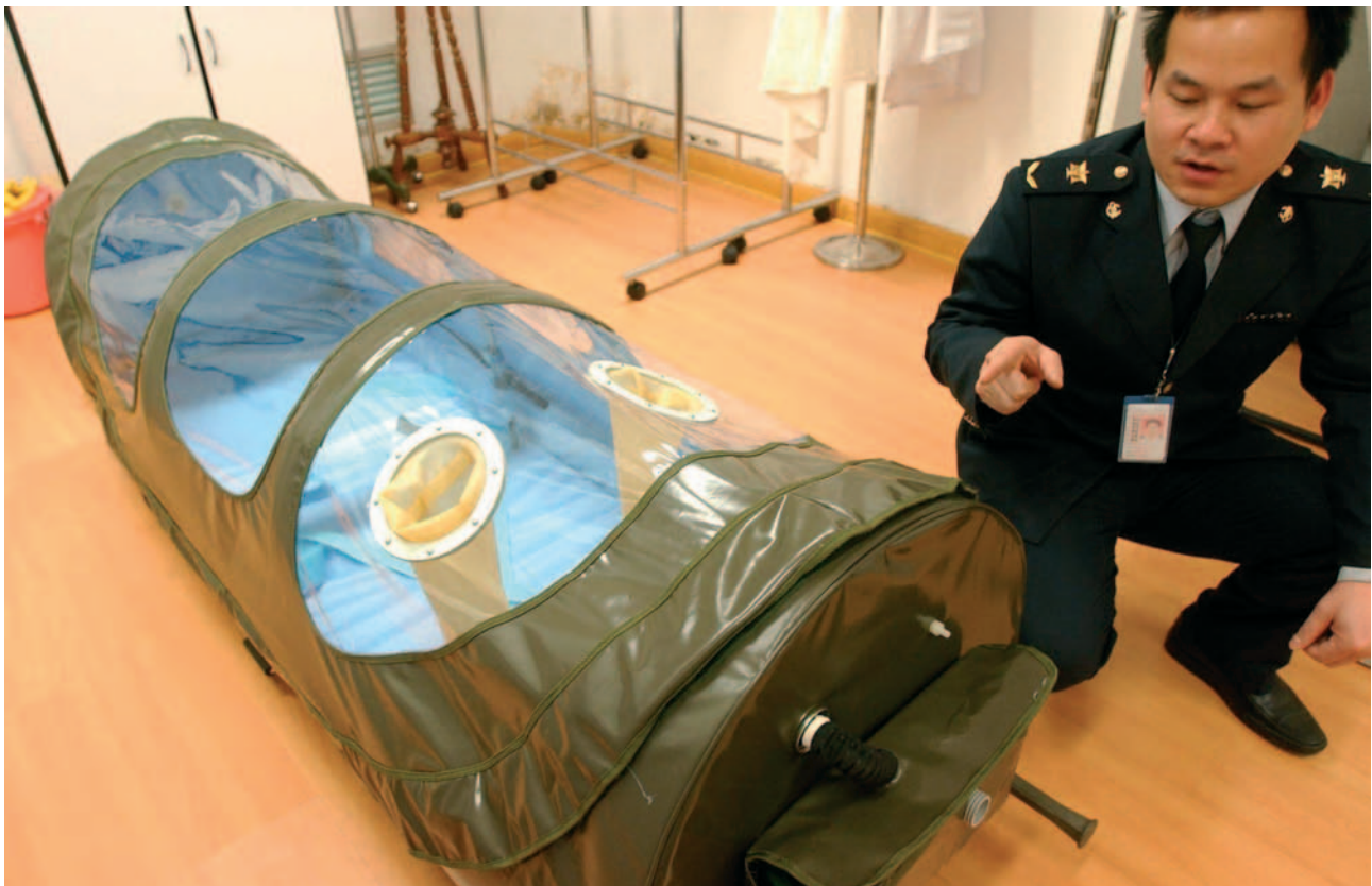
One of the enclosed beds designed to contain disease-infected travellers at the border checkpoint in Nanjing, China's eastern Jiangsu Province.
