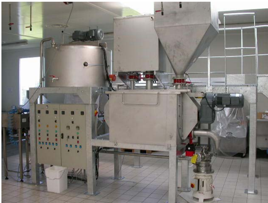
Single mixing/ packaging unit for large scale of RUTF
