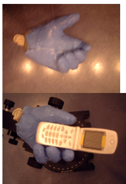
Fig. 1. Hand phantoms (a) Hand phantom A (b) Hand phantom B against phone
