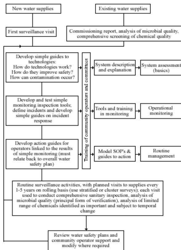
Figure 13.3: Implementing the water safety plan roll-out
