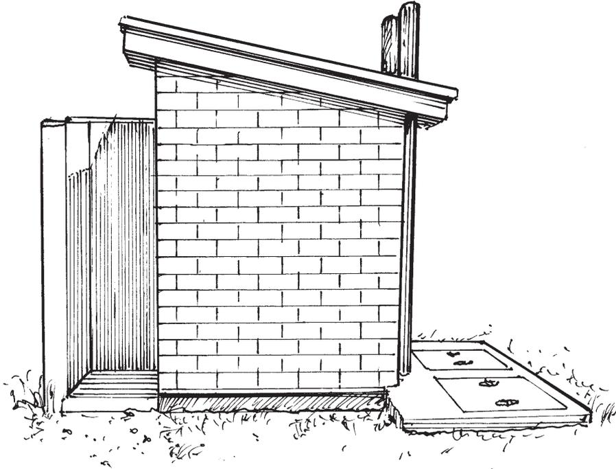
Figure 4.4 *VIP latrine*
