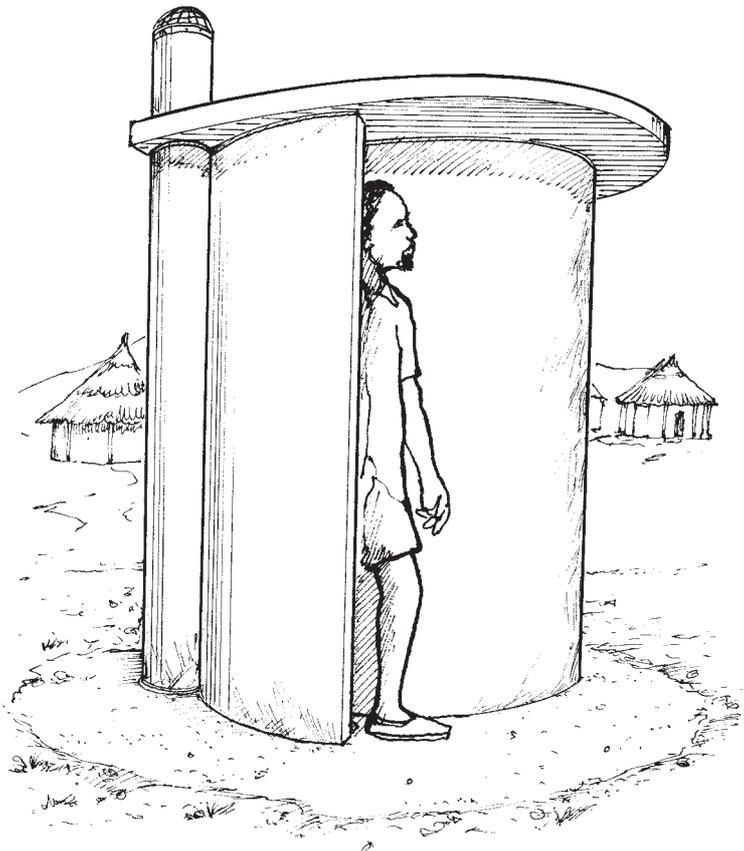
VIP latrines may be designed with single or double pits. Double pits may be used, for example, when cultural taboos prohibit the mixing of male and female faeces. Twin pits may also be used to facilitate emptying and composting. When one pit is full, the other can be emptied and reused. The pit of a VIP latrine is usually located directly beneath the slab to prevent fouling of the chute, which would lead to odour and fly problems, and require regular cleaning.
