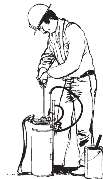
Fig. 9.12 Pressurizing the spray tank.
