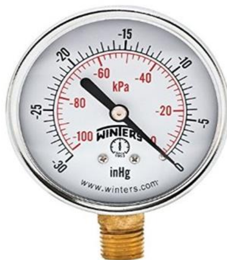
Figure 3. A pressure gauge reading from -100 to 0 kPa. In this case, the correct vacuum level for the test would be -80 kPa (red numerals).
